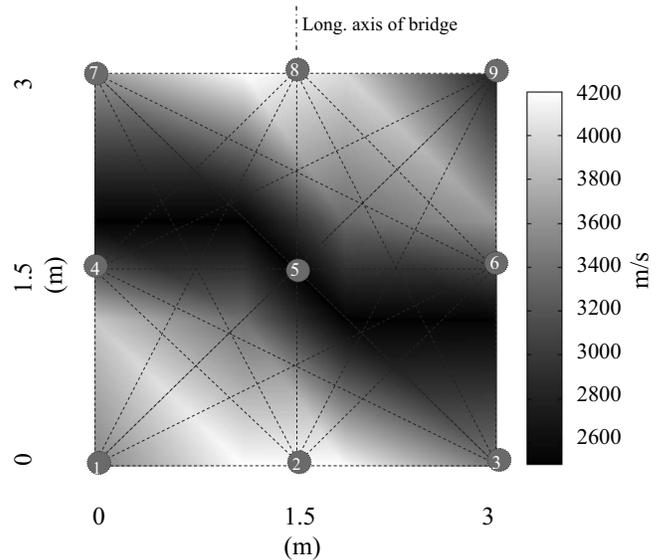
Fig. 6. Velocity structure of the bottom surface of the bridge concrete. The positions of the transducers are indicated by a closed circle, and the examined wave paths by dashed lines.
