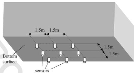
Fig. 5. Sensor arrangement for surface wave measurements
