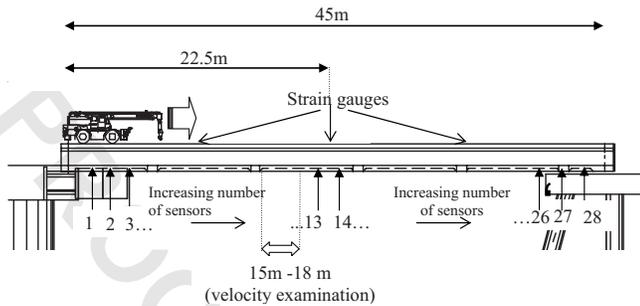
Fig. 1. Representation of the crane passing over the bridge and sensors location
